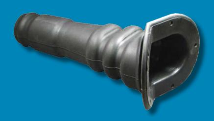
One of our most recent problem solving tasks involved designing a rubber boot for a steering column. The customer was unsure if the component could be made from rubber, and was told by other sources that the unique angle located at the base of the steering column would prevent the part from being molded. We knew better, and after discussing the project with their engineers, Ashtabula Rubber designed a molded component to meet all field requirements. Needless to say, our customer was satisfied.
